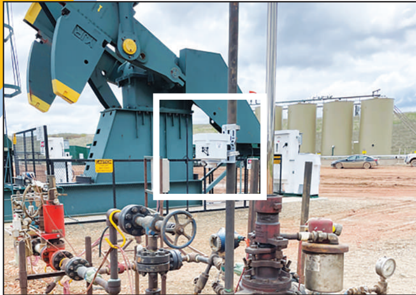
MethaneTrack™ endpoint in close proximity to compressor
