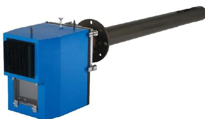
DGA-X model delivers reliable, precise performance at excellent value. It was proven UV-DOAS technology to measure SO<sub>2</sub>, NH<sub>3</sub>, separate NO & NO<sub>2</sub> measurement is possible through this technology. perfect solution for CEMS, FGD Inlet, Outlet. IT also has an option available with teflon coated probe. This model suited & proven in rugged application.
